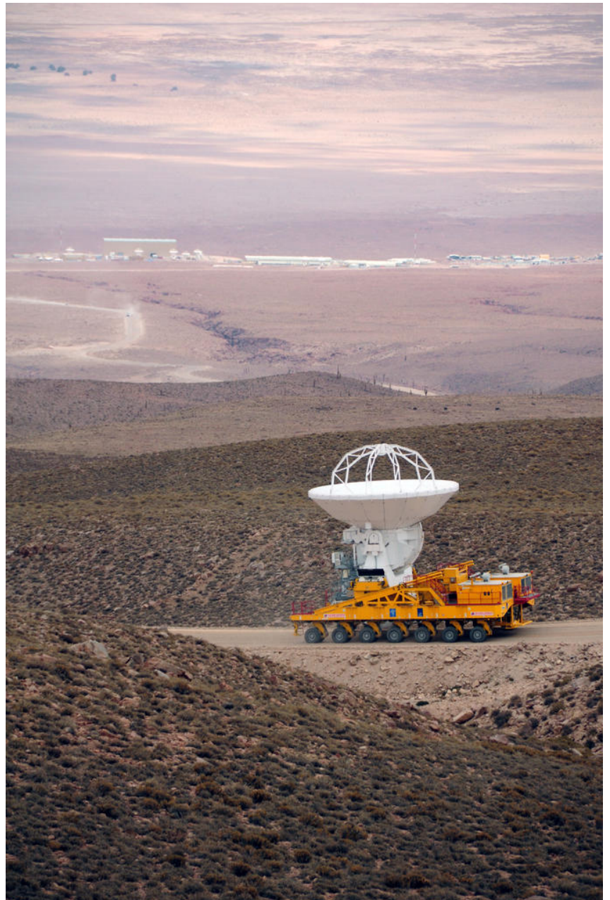
Figure 11: The first ALMA antenna was transported to the AOS on 17 September 2009. The transporter and antenna climb above 4000m, leaving behind the OSF and the 21km that separate it from the Chajnator plateau. © ALMA (ESO/NAOJ/NRAO)
